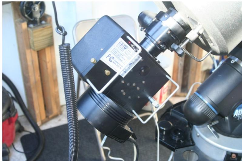
Fig. 1 SBIG Spectrograph mounted to a Celestron 9.25 telescope at Farm View Observatory.
